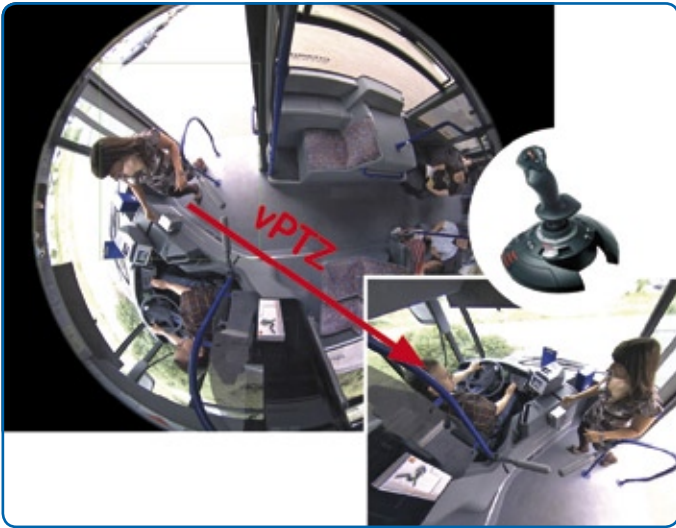
Virtual PTZ: The camera zooms in on detail. The image of the hemispheric camera can be enlarged and any image section examined using a joystick.
