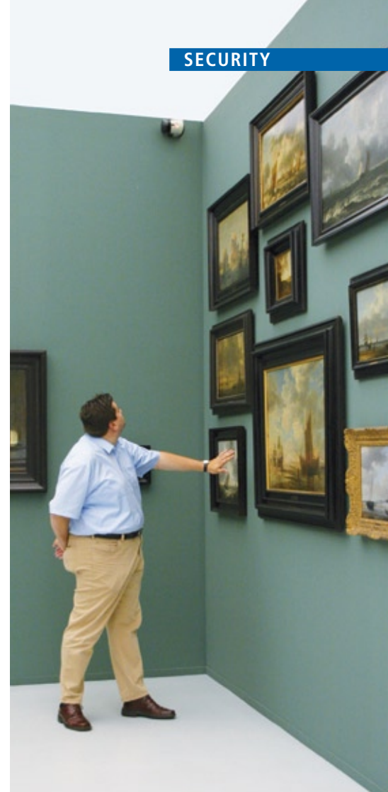
The time-of-flight of the emitted light pulses changes – leading to the triggering of an alarm signal by the LMS120 – as soon as a person reaches into or enters the protective field.
