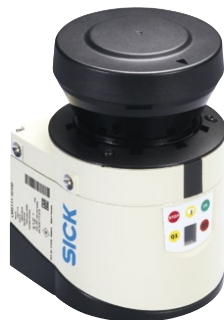
The actively scanning LMS120 transmits invisible fan-shaped laser pulses with an angular resolution of 0.25^\circ and scanning frequency of up to 50 Hz within a 270^\circ angle.
