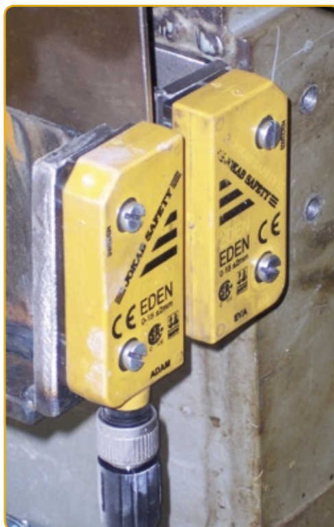
◀ Fig. 3: The Eden electronic safety sensors have a sensing distance from 0 to 15 mm. Thanks to their large tolerance for misalignment and offset their mounting is totally uncritical.
