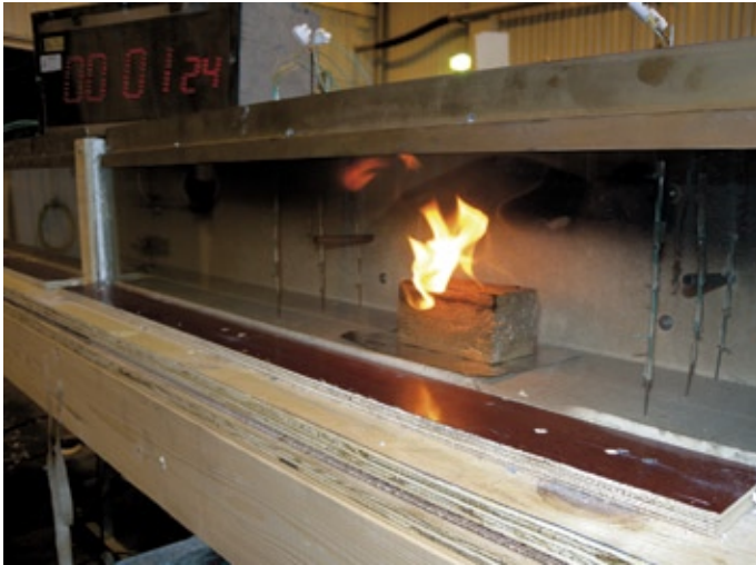
4 A Fire Test in a Model-scale Tunnel
