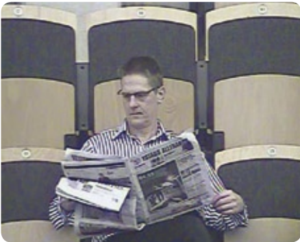
Fig. 1: Max. tele view with a 36x zoom, 4CIF camera
