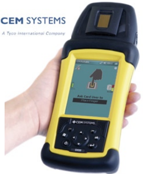
S3020f portable reader with up to 100,000 card and biometric records
