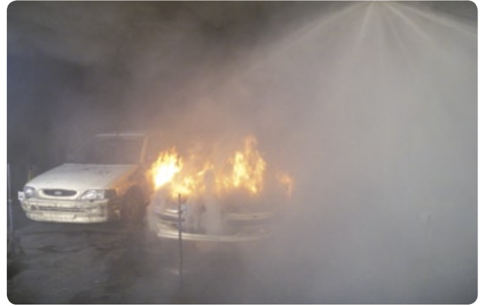
Test of water mist, immediately after activation of the first nozzle.
