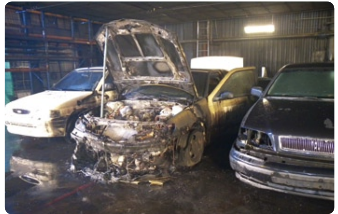
The fire damage after the test. All the tyres, the engine area and parts of the front of the car have been destroyed, but the system has prevented the fire from spreading to the adjacent cars.
