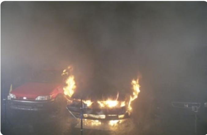
Test with traditional sprinklers about five minutes after activation of the first sprinkler. The direct wetting of the cars on each side prevents the spread of fire.
