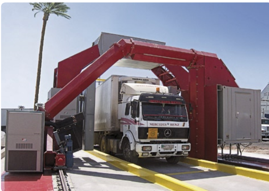
OmniView Gantry provides four views of the cargo. High-energy X-rays penetrate dense cargo. Z Backscatter highlights organic materials, with photo-like images from three-sides: left, top, and right.
