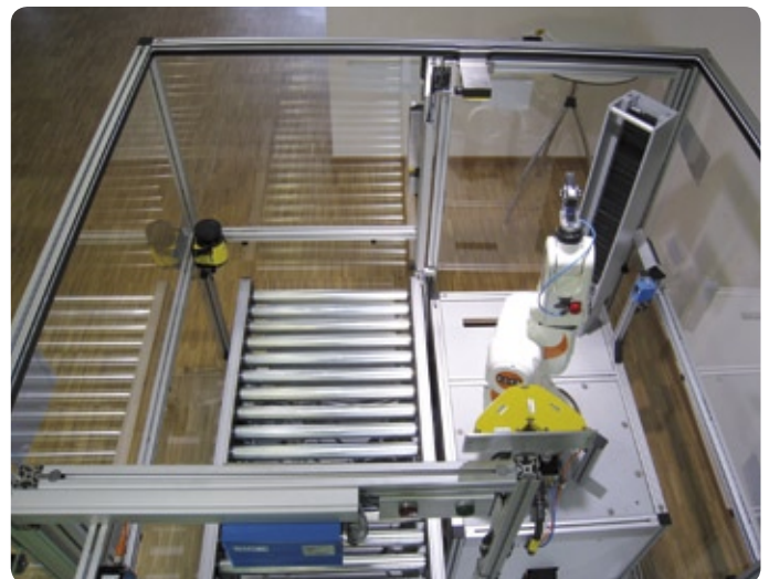
Turn key safety solution made by SICK including safety scanner S300 at conveyor and two safe vision sensors V300WS.
