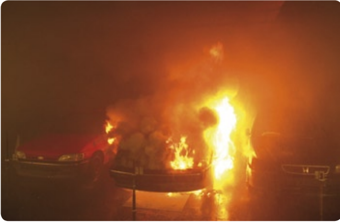
Test with traditional sprinklers just before the first sprinkler activated.
