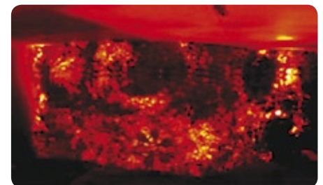
Hot spots in a waste bunker can lead to spontaneous self combustion and fires
