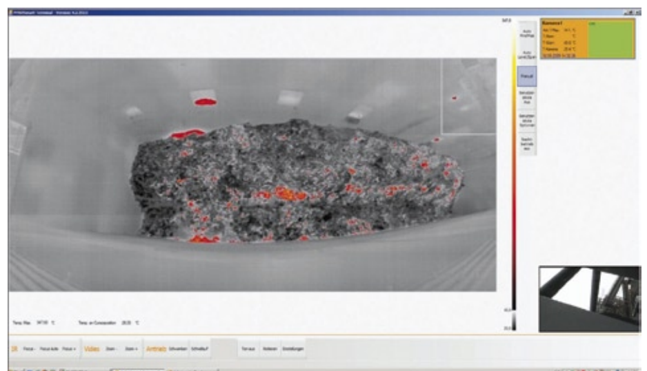
The PYROsmart system clearly shows the areas that are susceptible to spontaneous self combustion. The fire monitor will cool these areas down.
