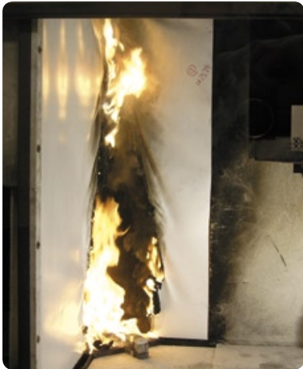
Fig. 2a: SBI testing of a textile membrane
