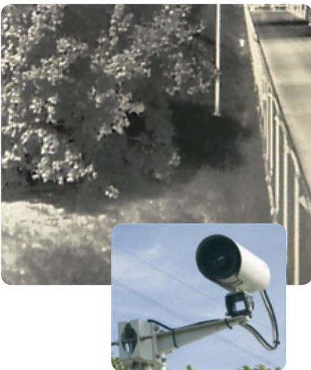
Branches moving in the wind caused many unwanted alarms in this location, so Krüger decided to replace the CCTV camera with a thermal imaging camera. Not one unwanted alarm has occurred since.
