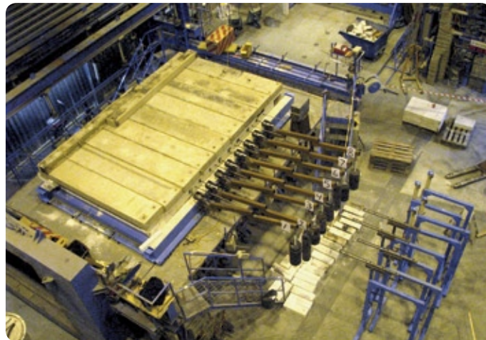
Fig. 4b: The top view of the furnace with load arrangements and strain gauges
