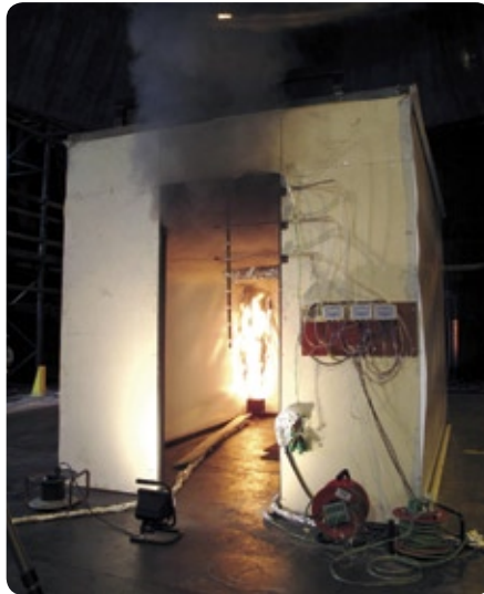
Fig. 2b: Largescale reference test using textile membrane
