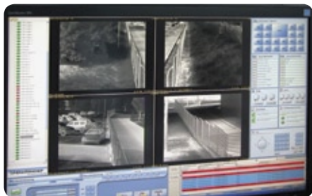
Visual analysis software is much more effective when connected to thermal imaging cameras. "A trespasser shows up very distinctly due to the thermal contrast", explains Krüger.
