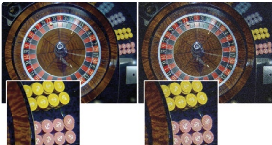
Sample images with high noise (right) and low noise (left). Under low light conditions, images from sensors with small pixels may exhibit more noise than those with large pixels.
