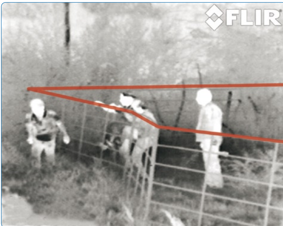
The Flir Sensors Manager Pro software includes an advanced video analytics module. The user can place virtual trip wires and other triggers. A silent alarm will go off if someone crosses the trip wire.
