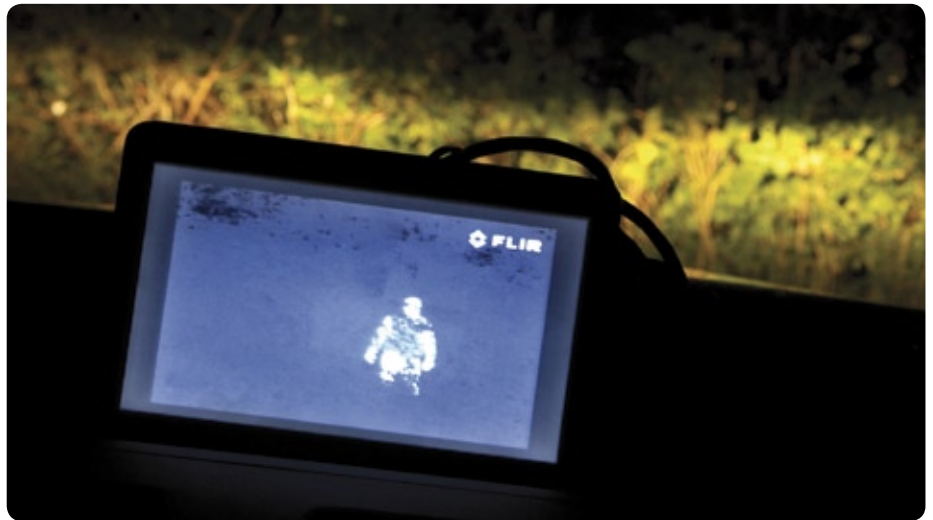
The high contrast thermal footage is displayed on a TFT screen on the dashboard.
