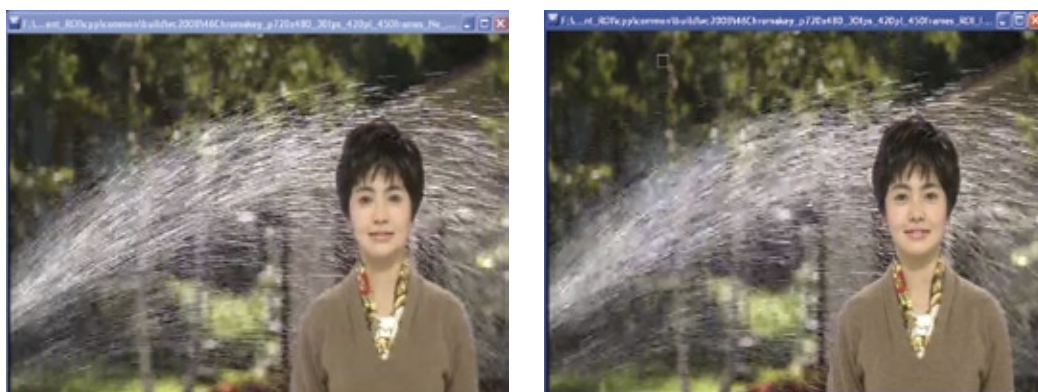
Chroma-key sequence, H.264 encoded at a low bit-rate in order to stress the VQ difference. (left) No ROI applied. (right) ROI applied.
