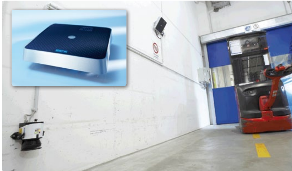
The RFU630 interrogator with UHF technology and a scanning range of 5 m offers the highest security in long-range identification of transponders especially for intralogistics applications.
