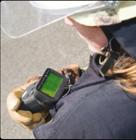
Was the winner in 2009 of the GIT SECURITY AWARD and is standard equipment for many monitoring tasks: Microtector G460 7-gas measurement device in use here with the fire brigade.
