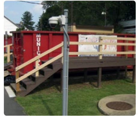
A panoramic camera watches out for illegal dumping at a waste center
