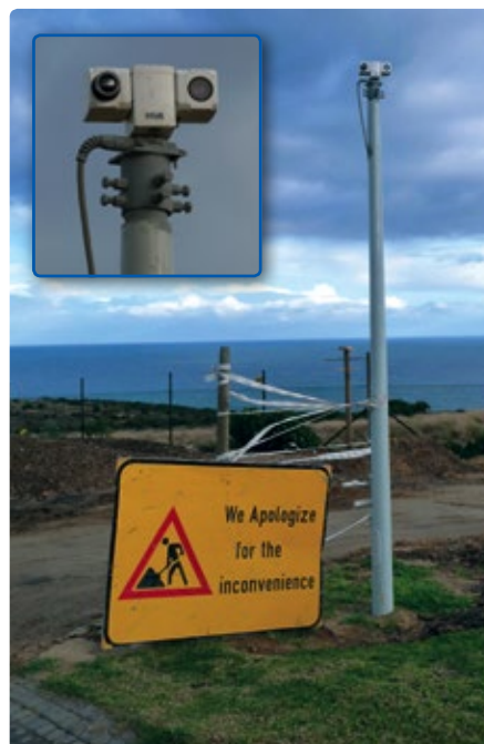
One of the Flir Systems PTZ-50 MS thermal imaging cameras overlooking Oubaaï.
