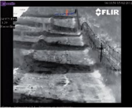
Human targets are being tracked and will trigger the alarm when crossing the virtual fence
