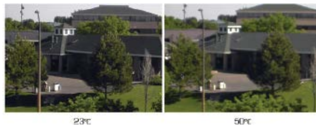
How the focus varies when a temperature change occurs after installation
