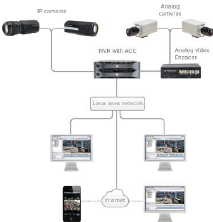
With the Avigilon Control Center and High-Definition Stream Management security officers have access to all cameras on very little bandwidth
