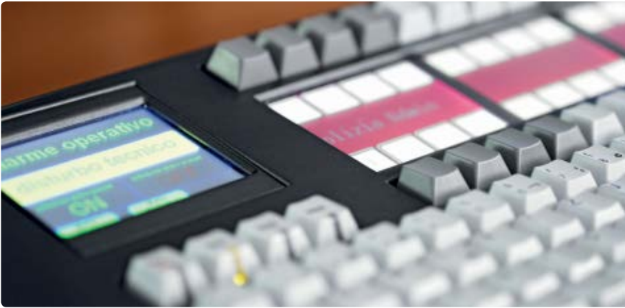
Alarms, system reports, failures etc. are automatically displayed at the workstation and/or on a large scale video display
