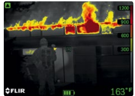
▲ TI Basic mode: For initial size-up of fire scene and fire attack
