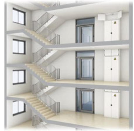
To ensure a safe escape in case of a fire, stairways that serve as rescue routes should be separated from the rest of the building in a fireproof construction
