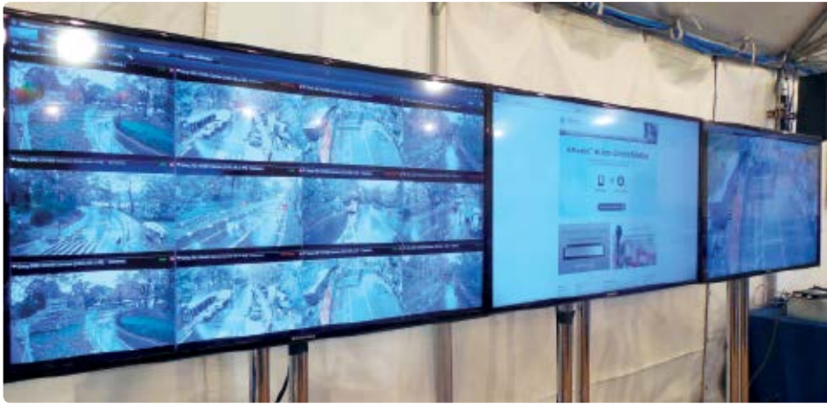
At the Race Command Center a XProtect Smart Wall displayed 36 simultaneous camera views
