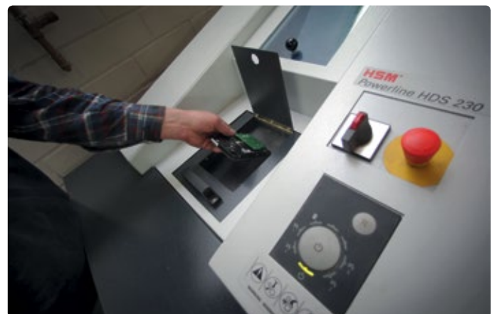
The Powerline HDS 230 from HSM will correctly destroy magnetic and optical storage media
