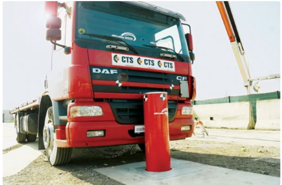
▲ Proven to defy 7.5 tonnes – an PPG crash bollard
