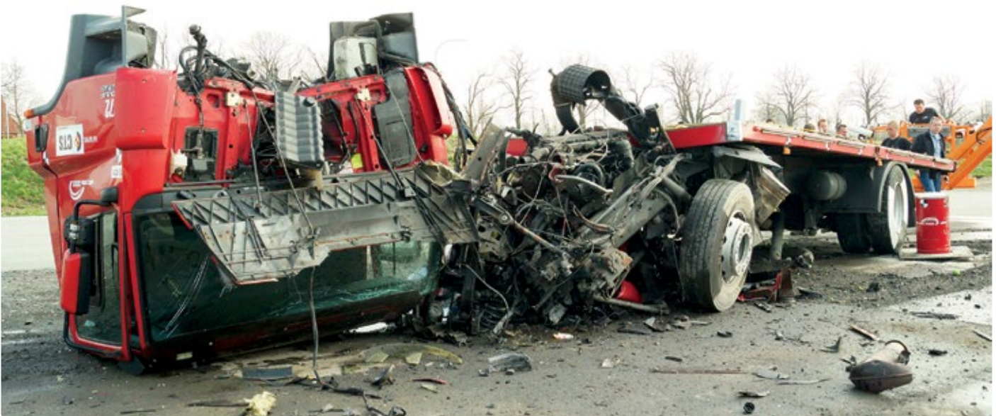
▼ A truck after a crash test against a hydraulic PPG M50 barrier
