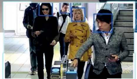
FACE ORIENTATION: ANGLED FACES Horizontal range : \pm 45^\circ Vertical range : \pm 30^\circ
