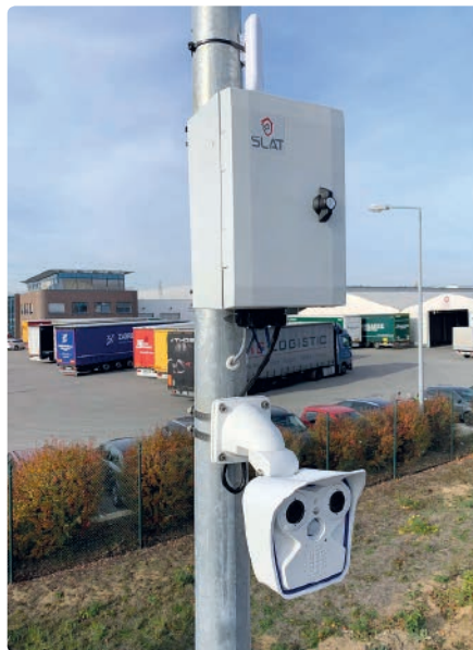
All-in-one solution for secure video surveillance. An outdoor network interface box with attached day/night camera and WLAN bridge
