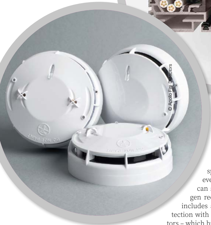
▲ The Soteria Optical/Heat Multisensor Detector uses new optical sensing technology, PureLight, to detect smoke particles entering the chamber and is fitted with two thermistors for detecting heat
