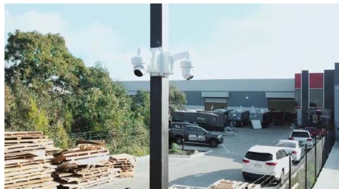
Complete coverage of the perimeter is provided by ten Hikvision cameras with smart event detection technology
