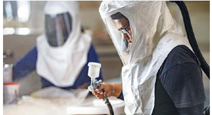
Yugeshni Naidoo is wearing a Dräger X-plore 8000 Powered Air Purifying Respirator combined with a hood worn over a bump cap thus protecting head and eyes.
