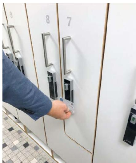
The ‘Z lockers’ have been converted from mechanical locks to an RFID solution with a time-limited period of use
