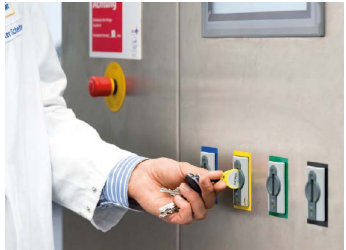
Ritter Sport's raw ingredients are unloaded at the right receiving station and into the right container via a programmed EKS chip
