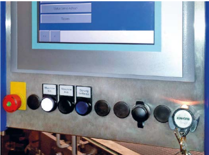
The modular Electronic-Key adapter for the EKS Light can be seen on the right-hand side of the operating unit
