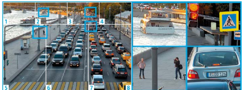
Multifocal sensor technology is particularly well suited for urban surveillance: even in complex locations, a high-resolution overall view is always available, even in recording. At the same time, operators can open a theoretically unlimited number of detail zooms in parallel ('virtual PTZs')
