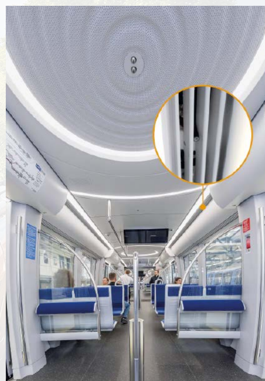
The air sampling points of the Titanus aspirating smoke detector are discreetly integrated into the car and are virtually invisible
