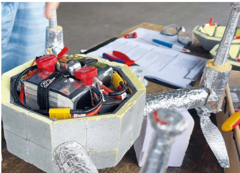
Glass fiber-reinforced aerogel surrounds the heart of the drone and protects the power supply and the electronics from heat
