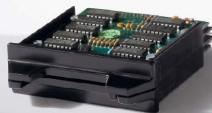
Interflex developed a fraud-proof and patented infrared card reader at the time that was built into all time recording and access control solutions as from 1977
