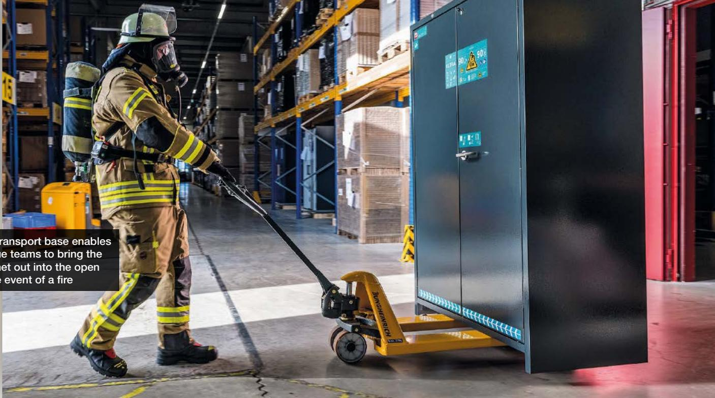
The transport base enables rescue teams to bring the cabinet out into the open in the event of a fire
