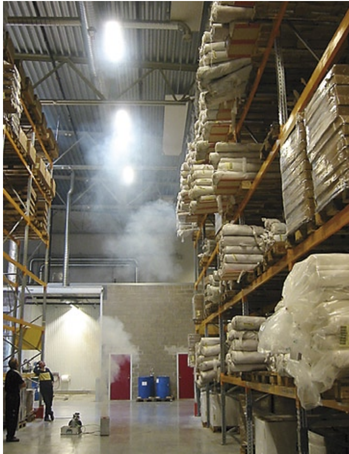
It is not certain that the smoke from a small fire will reach all the way up to the ceiling in a high building.
