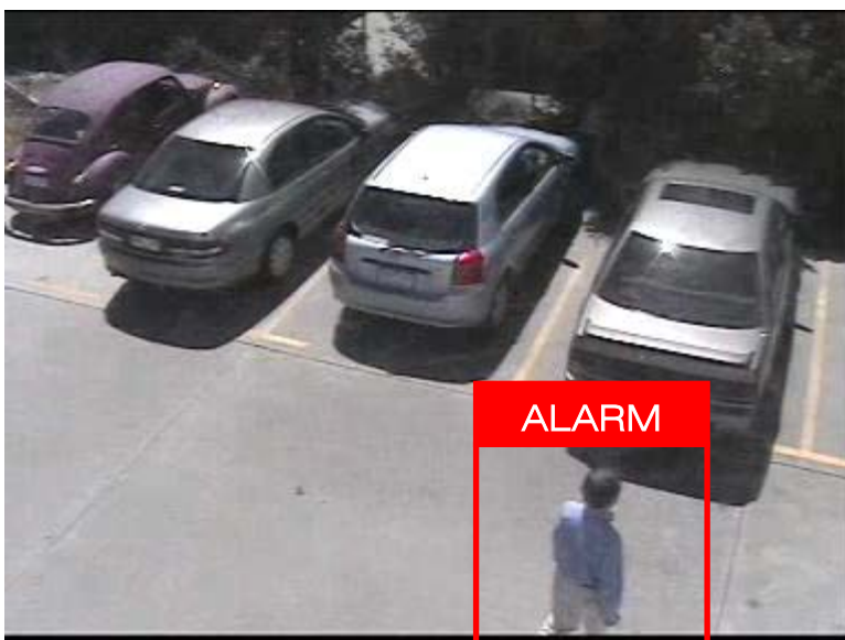
Intruder appears and is recognised by the VMD due to the change in pixels and recording begins.
